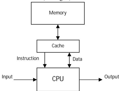
Fig 2: Modified Harvard Architecture
